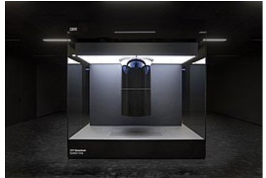
IBM Q System One, a quantum computer with 20 superconducting qubits [1]
