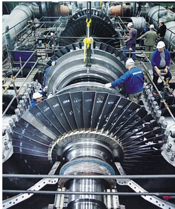
A steam turbine with the case opened, an example of energy technology
